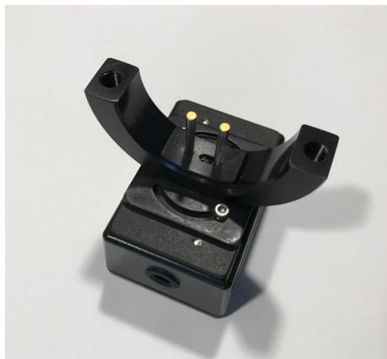
The pressure-sensing (-PSO) option for the CDI 5100, 5200 & 5400 flowmeters allows plant managers to monitor pressure throughout an air distribution system along with flow. For the 5200 & 5400 meters, the pressure sensor is mounted next to the flow-sensing probes. It accesses pipe pressure through a cutout in the gasket that seals the ring to the pipe. For the 5100, the pressure sensor is mounted in the top plate. In either case, there are no additional steps during installation.
